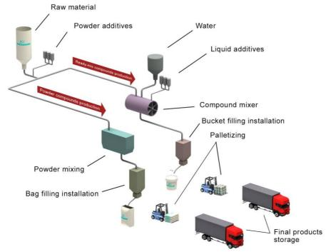
Raw materials are received in the manufacturing plant, where they are weighted and mixed according to the formulation. Once raw materials are mixed, the product is packaged in bags for its storage in pallets until the product is distributed.
