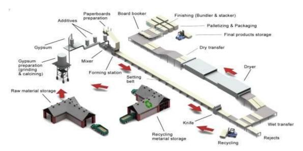
Raw materials are homogeneously mixed in the mixer to form gypsum plaster, which is discharged through output pipes on a paperboard sheet that is advancing on the forming belt. In parallel, a second paperboard sheet is added to form the Laminated Plasterboard. The board continues advancing on the production line until it acquires enough hardness to be cut. It is subsequently dried in a continuous process. Finally, it is stacked, palletised, and shrink-wrapped to form the packaged product.
