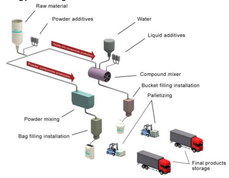
Raw materials are received in the manufacturing plant, where they are weighted and mixed according to the formulation. Once raw materials are mixed, the product is packaged in a plastic bucket for its storage in pallets until the product is distributed.
