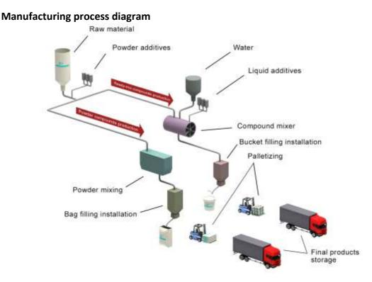
Raw materials are received in the manufacturing plant, where they are weighted and mixed according to the formulation. Once raw materials are mixed, the product is packaged in bags for its storage in pallets until the product is distributed.
